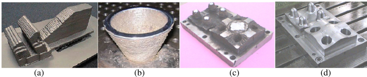
Fig. 22 a As deposited sample made by wire-feed LAM (AeroMet), b thick wall structure produced by hybrid layer manufacturing (HLM), c near-net shape of the die pair and d finished die pair produced by HLM [29]
