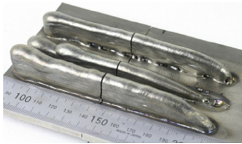
Fig. 19 Thin walls built by weld deposition showing the changing bead geometry at the start and end portions [70]
