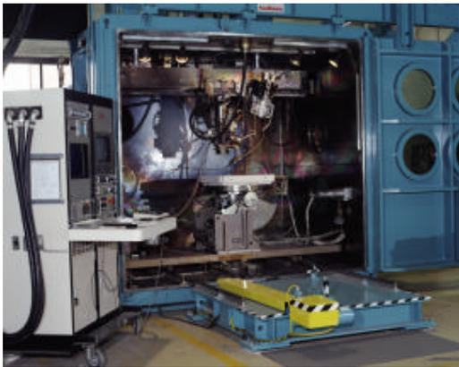
**Figure 2. Ground-based EBF<sup>3</sup> system at NASA Langley Research Center.**
