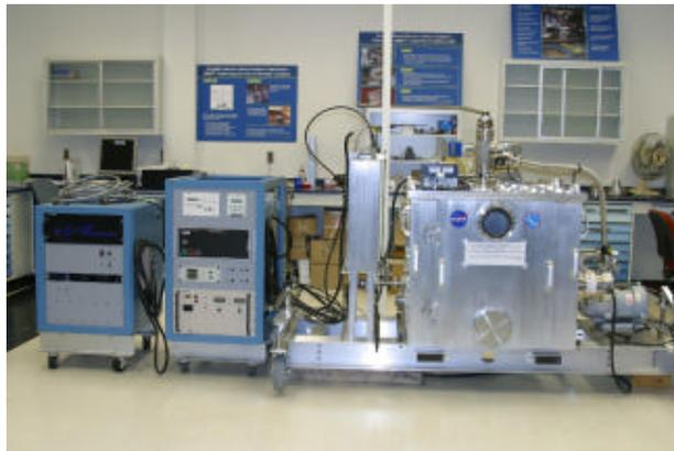
**Figure 3. Portable EBF<sup>3</sup> system at NASA Langley Research Center.**
