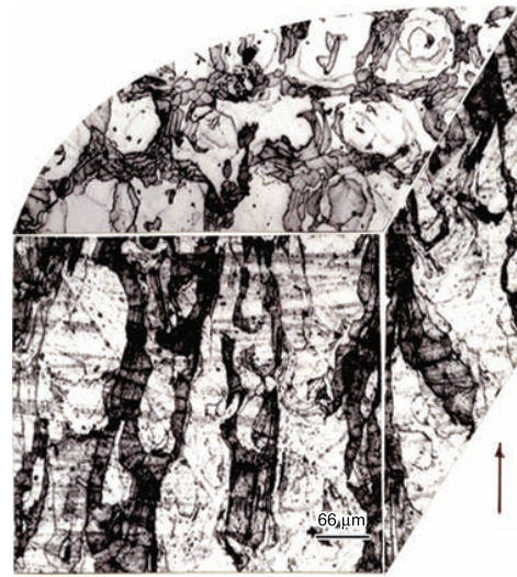
Fig. 16 3D-optical micrograph composite section view for 17-4PH stainless steel nitrogen atomized powder fabricated in argon gas ( \text{N}_2\text{-Ar} ) fabricated by SLM. The build direction is shown by arrow at lower right
