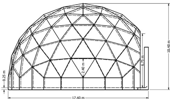
Fig. 2. Agriculture/construction dome diagram.
