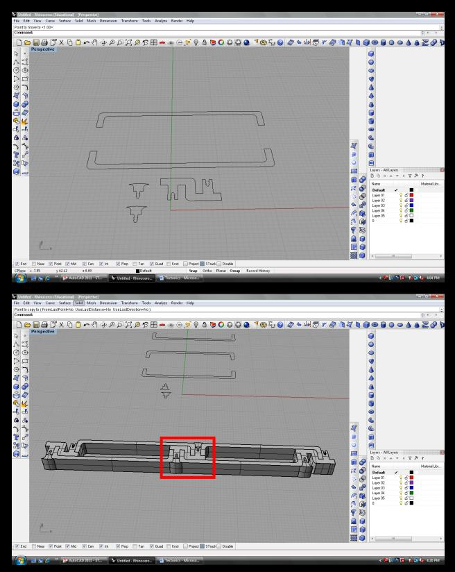
This is an issue with glass panels. The support / connection will not be translucent. This type of connection would be better for aluminum wrapped insulated panel.
