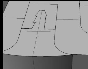
Once the pieces were printed I discovered I needed a tolerance, or at least on the BFB 3000. I also noticed that due to possible temperature factors the print was warping.
