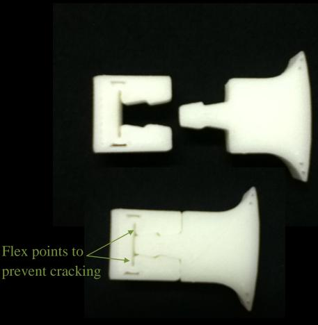
I scaled the project down for shorter print times and because my focus was merely to define a perfect tolerance for connections on the RapMan 3.1. I also went with a single gripping element for this application.
