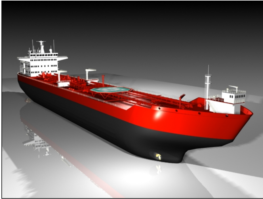
Figure 8 – 70,000 dwt Tanker for Russian Arctic – Twin Azipod Propulsion
