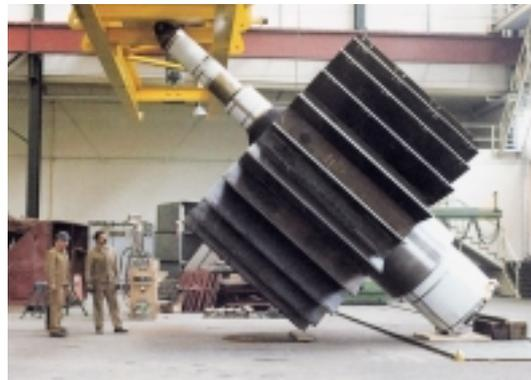
Inner rotor for a large APH before shipping
