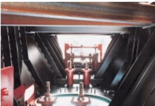
Radial seal adjusting device
