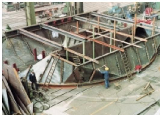
Concentric APH: Manufacturing of connecting ducts
