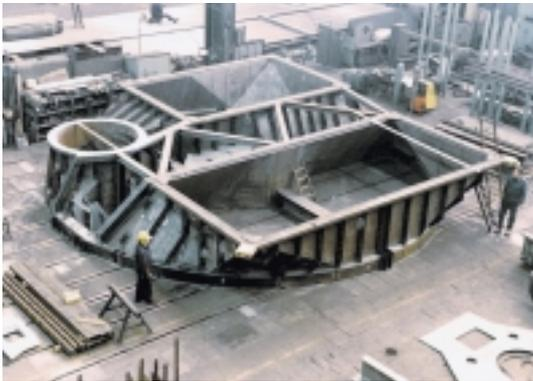
Tri-Sector APH: Workshop assembly of connecting ducts
