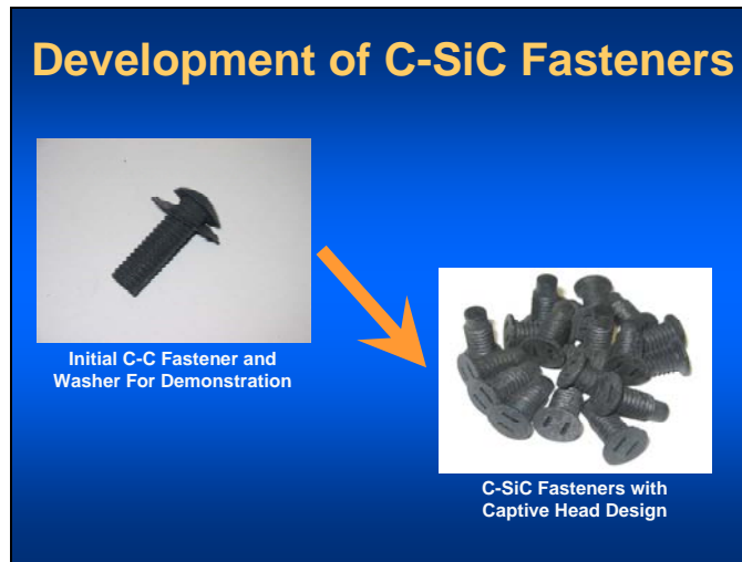
Figure 34. R&D development of C-SiC fasteners to be used alone (to plug small hole damage and/or in conjunction with the small- and large-area repair concepts (SAR and LAR)).
