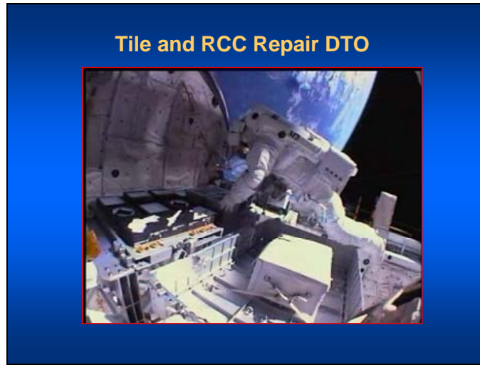
Figure 26. EVA astronaut Steve Robinson demonstrating several tile and RCC TPS repair techniques in the payload bay during STS-114.
