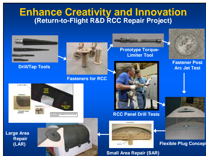
Figure 29. Some of the tools developed for on-orbit RCC repair by the R&D RCC Repair Team.
