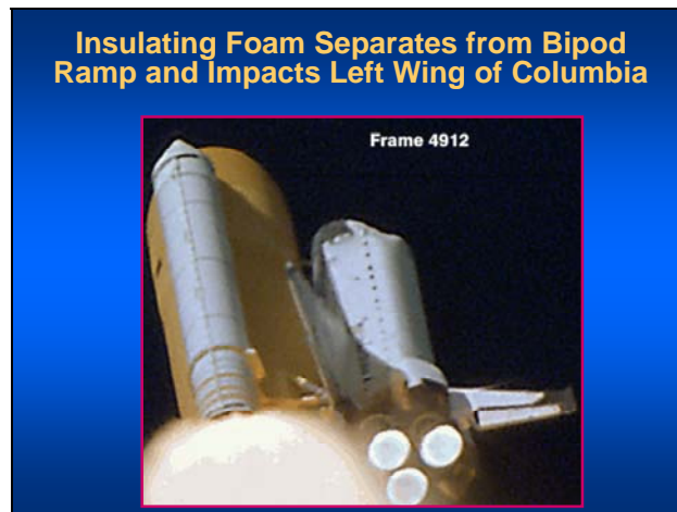
Figure 2. Launch video of STS-107 illustrating the impact of a large piece of external tank (ET) foam hitting the lower surface of the Orbiter.
