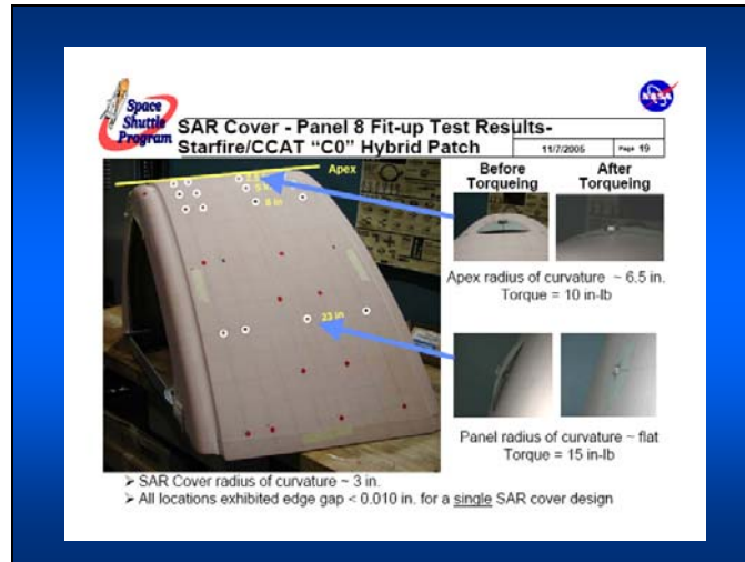
Figure 39. Fit check of the R&D RCC Repair Team's 4-inch diameter doubly curved, C-SiC small area repair (SAR) concept on the most highly curved Orbiter RCC leading edge.
